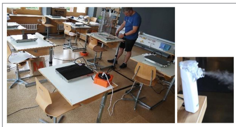
Figure 6: Salt Aerosol Generator and Hot Plates in The Classroom Simulating the Body Heat.
