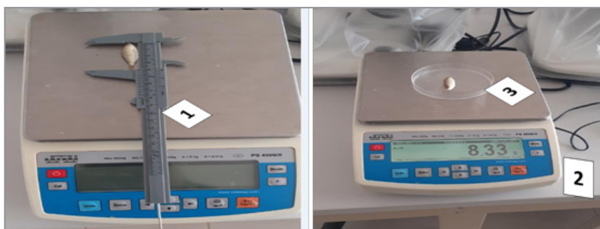
Figure 6: Biometrics of juveniles at the end of the experiment, with ichthyometer (1), precision scale (2) and Petri dish (3). Source- Personal archive.
