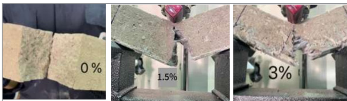
Figure 9: Fracture of composite specimens
