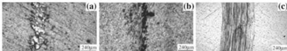
Fig. 8 Wear surface morphology of a Nitriding after molybdenizing and b molybdenizing for 200 m and c Ti6Al4V for 100 m
