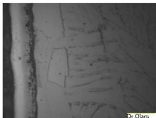
Fig. -- Sectional microstructure of Mo-alloyed layer on TC4 substrate
