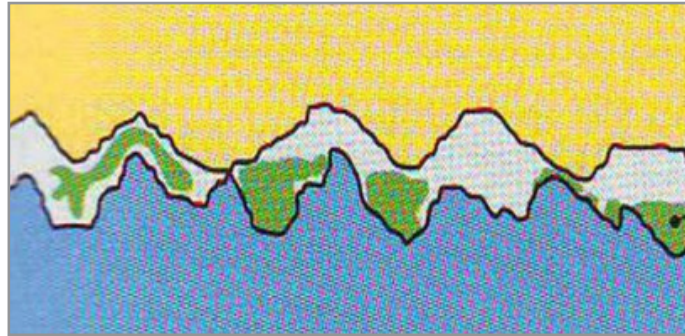
Figure 5: Schematic of a rough contact
