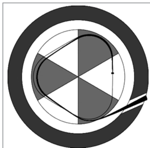
Figure 5: The extraction of the 15 MeV proton beams due to 5% energy losses at the degrader.
