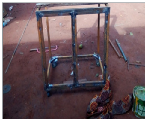
The 1-inch Iron Pipe Was Welded Together to form a Framework for the Cabinet
