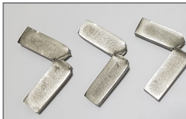
Figure 6: specimens conducted - V impact test
