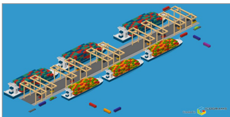
Figure 5: The Floating Terminal Design Configuration
