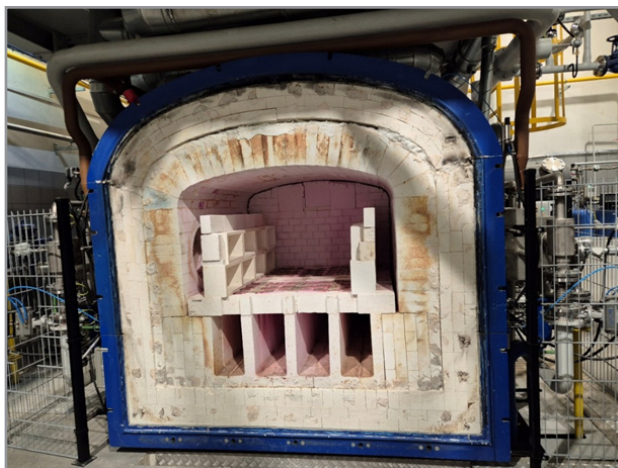
Figure 2: Photograph of a hydrogen-fired furnace at Łukasiewicz-ICiMB
