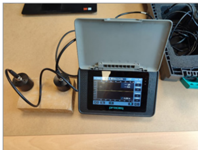
Figure 2: Pundit PL-200 Proceq instrument and Compressed Earth Block (BTC).
