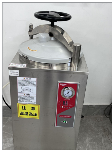
Figure 1: Healthy Soil Placed in Vertical Steam Pressure Sterilizer to kill Microbial Communities
