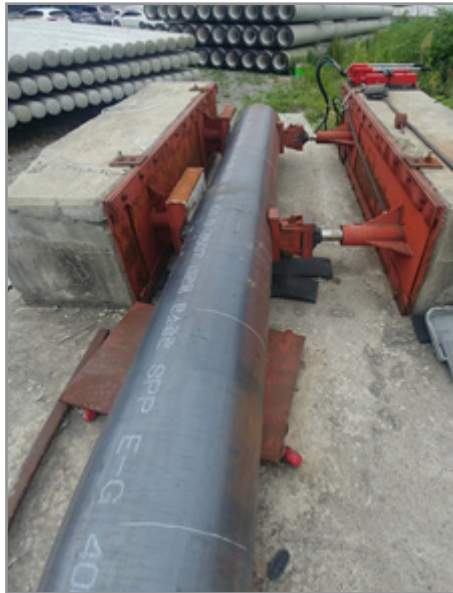
Figure 12: Boundary conditions for performance testing (fixed end)
