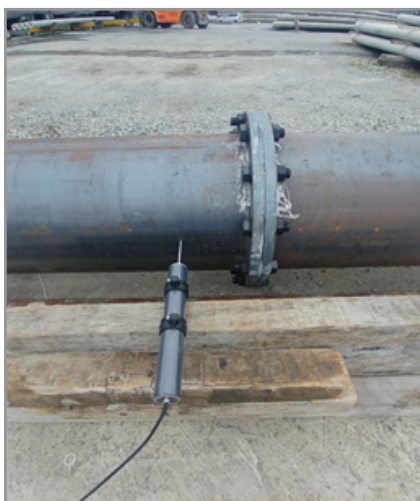
Figure 14: Straight displacement transducer installed externally
