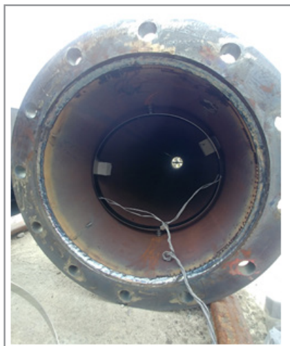
Figure 13: Installation of circular displacement transducer
