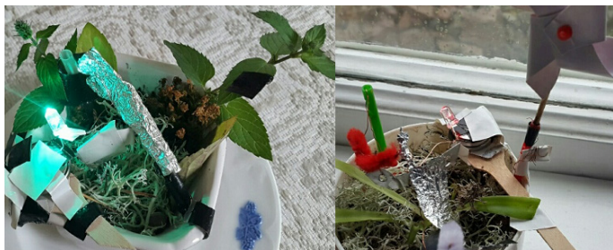
Figure 2: Two plant-lamps with Al-foil capacitors attached as in the scheme Figure 1. At right, a more rigid plate strip in the capacitor.
