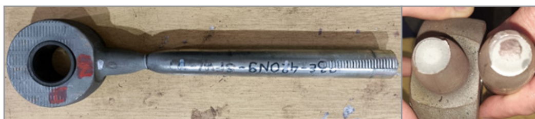
Figure 2: Fractured spindle after tensile testing
