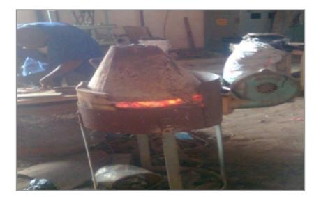
Casting: when the metal had become molten, it was removed from the furnace. Some quantities of slag or impurities were removed to obtain the pure metal and were poured on the mould; the mould was allowed to solidify for some minutes. A casting was formed.
