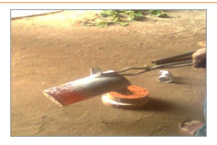
Fettling: The casting was taken to fitting shop for fettling cutting of the ingate and file to size using hand file and sand paper [6].
