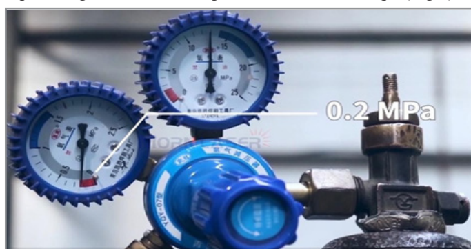
Fig 5: The required gas of the laser welding machine and its pressure.
