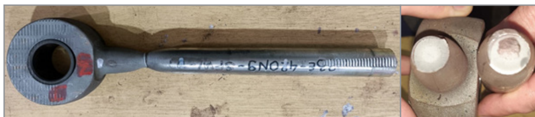
Figure 2: Fractured spindle after tensile testing
