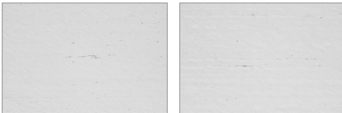
Figure 3 (a and b) Non-metallic inclusions in the both parts of the spindle
