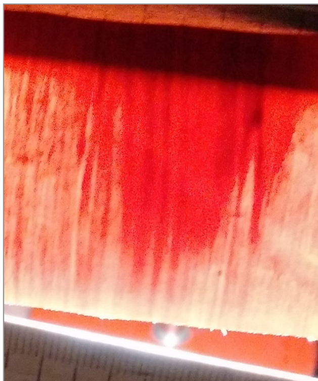
Figure14: Diffraction Lines; Sample-W Foil (Double Cylinder). Photoexcitation (250nm) ~ 15min 14 days. Horizontal Position of “Photo Paper” with HgS, on the SGK
