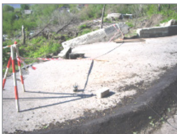
Figure 2: Installation of a mobile system for dynamic and geophysical monitoring of a landslide-prone section of the road in Ulyanovsk
