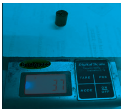
Figure C.1.1.2. Post pellet drying and firing weighing.
