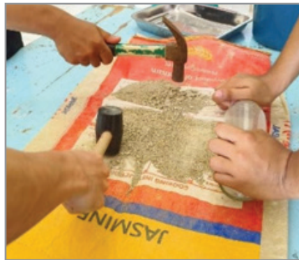
Figure B.1.1. Clay sample preparation: pulverizing.
