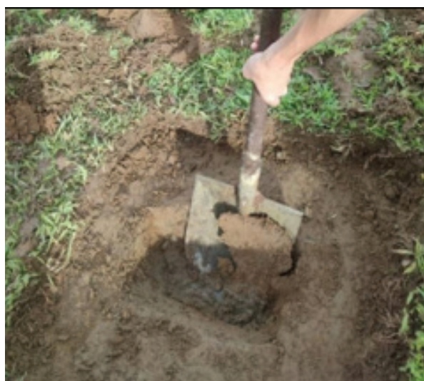
Figure A.1.2. Scraping and Trenching to access the upper layer of prospected clay deposit.
