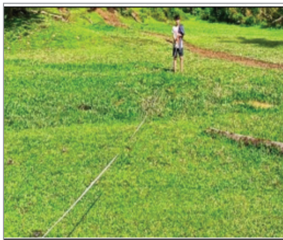
Figure A.1.1 Performing Composite Sampling Method (zigzag pattern), 10 sampling points with a regular interval of 10 meters.
